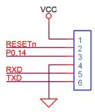
The ISP function uses only six pins: VCC, GND, RXD, TXD, P0.14 and RESETn. The simple circuit above is all that must be added to the user's application to use ISP with USB-ICP.
