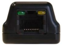
USB-ICP uses a standard RJ-45 for connection to the target cable.
