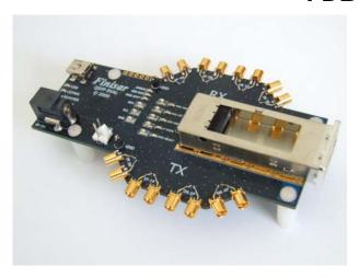
Finisar's FDB-1042 QSFP+ Evaluation Board is designed for testing and evaluating the QSFP+ transceiver and Quadwire<sup>™</sup> Active Optical Cables.
