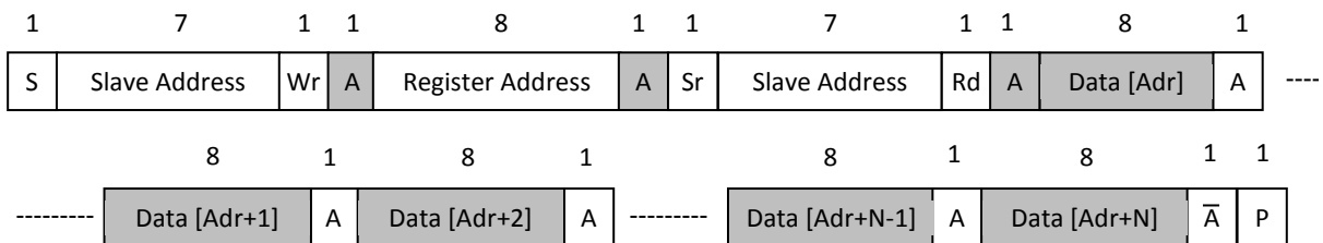
Figure 10: Register read format
