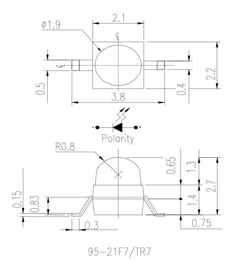
Note: The tolerances unless mentioned are  $\pm 0.1$ , unit=mm.
