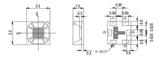
For Reflow Soldering(Propose)
