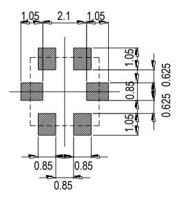
Note: Tolerances unless mentioned  $\pm 0.1$ mm. Unit = mm Suggested pad dimension is just for reference only. Please modify the pad dimension based on individual need.
