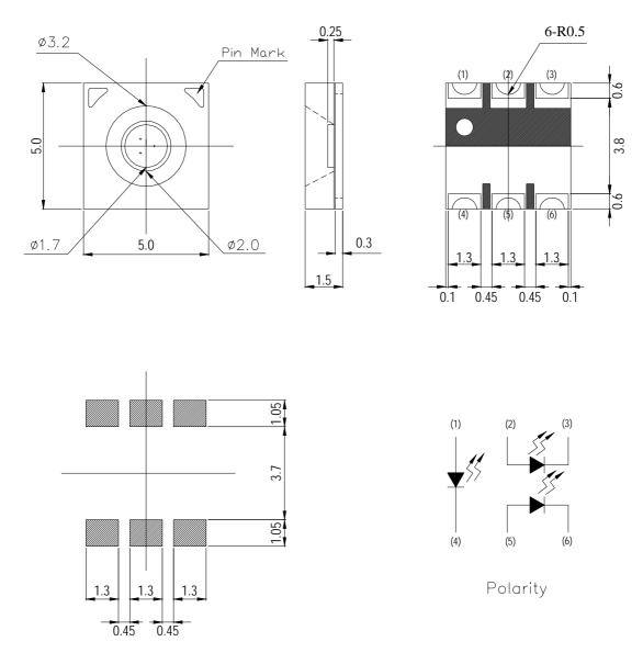
For Reflow Soldering(Propose)
