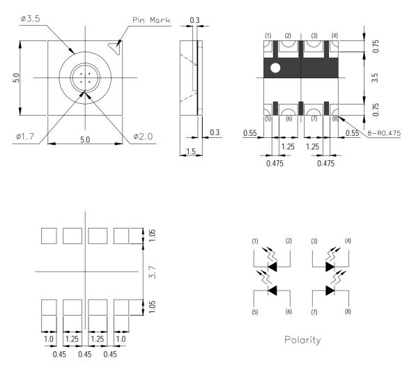
For Reflow Soldering(Propose)
