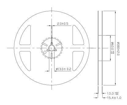
**Note:** Tolerances Unless Dimension ±0.1mm,Unit = mm
