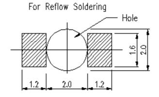
**Note:** The tolerances unless mentioned is  $\pm 0.1$ mm ,Unit = m
