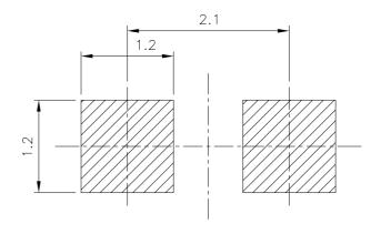
**Note:** Tolerances Unless Dimension  $\pm 0.1$ mm, Unit = mm
