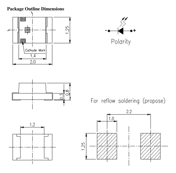
**Note:** The tolerances unless mentioned is  $\pm 0.1$  mm, Unit = mm
