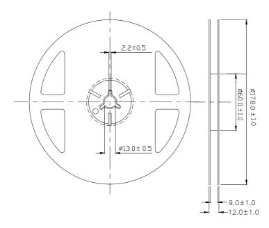
**Note:** The tolerances unless mentioned is  $\pm 0.1$  mm ,Unit = m
