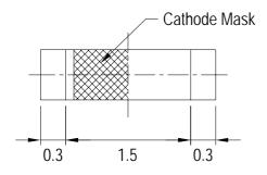
**Note:** The tolerances unless mentioned is  $\pm 0.1$ mm, Unit = mm
