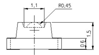
For reflow soldering (propose)
