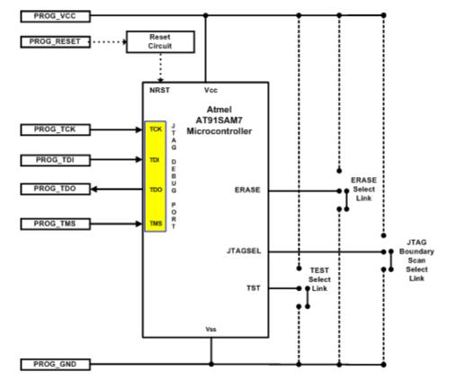
AT91SAM7 ISP Connector Cables for portable programmers
