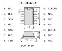
The metal case inside of the molding compound may be exposed on the top or bottom of this product. This purely cosmetic and does not have any effect on quality, reliability or electrical spoes.
