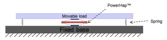
By applying a voltage to the actuator, it elongates and therefore moves the load. This movement can be felt by the user. For a maximal haptic feedback, the rear panel needs to be as heavy as possible. Otherwise the PowerHap<sup>™</sup> actuator will not only move the load but also the rear panel and therefore a part of the performance is lost.
