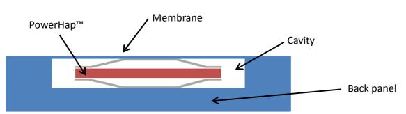
In this case the PowerHap<sup>™</sup> actuator is clamped between a thin, flexible membrane and a rigid back panel. By applying a voltage, the actuator elongates and consequently deforms the membrane.
