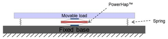
By applying a voltage to the actuator, it elongates and therefore moves the load. This movement can be felt by the user. For a maximal haptic feedback, the rear panel needs to be as heavy as possible. Otherwise the PowerHap<sup>™</sup> actuator will not only move the load but also the rear panel and therefore a part of the performance is lost.
