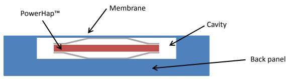
In this case the PowerHap<sup>™</sup> actuator is clamped between a thin, flexible membrane and a rigid back panel. By applying a voltage, the actuator elongates and consequently deforms the membrane.
