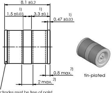
Electrodes must be free of paint material Cu-OFE - R200
