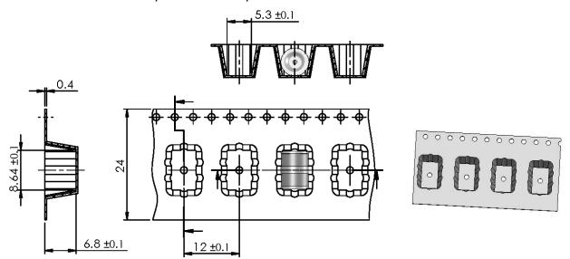
Tape and reel packing comply with the specification of IEC 60286-3
