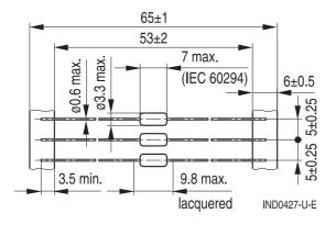
Minimum lead spacing 10 mm
