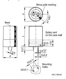
Snap-in terminals, length (6.3 + 1/-1.4) mm. Also available in a shorter version with a length of (4.5 - 1.4) mm. PET insulation cap is positioned under the insulation sleeve.
