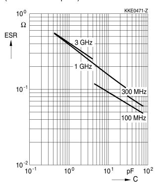
ESR versus capacitance C at self-resonant frequency (for soldered parts)
