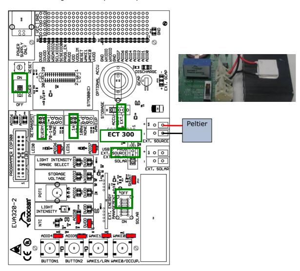
If heat sink has room temperature (e.g. 20°C) and you press one finger on the Peltier element above, the element will generate a few mV. ECT 300 will transform this to higher voltage and load short term capacitor on EVA 320. STM 300 will be powered by this energy and send telegrams.
