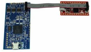
Use a debugger and JTAG adapter of your choice which supports the Cortex-M3 ARM core and more specifically the NXP LPC1343 microcontroller. You might need an adapter such as the <u>10-pin to 20-pin JTAG Adpater Kit</u> between your JTAG solution and the target board.
