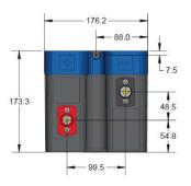
Positive Terminal: 5/16" – 18 threaded stud Negative Terminal: 3/8" – 16 threaded stud
