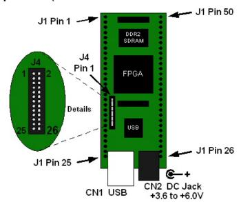
Simply connect the DLP-HS-FPGA to the PC to initiate the loading of USB drivers. Once the USB drivers are loaded, the DLP-HS-FPGA is ready for use. All commands are issued as multi-byte command packets consisting of at least two bytes.
