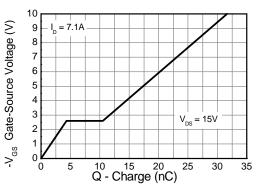
Gate-Source Voltage v Gate Charge
