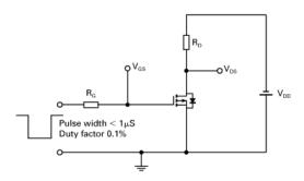
Switching time waveforms
