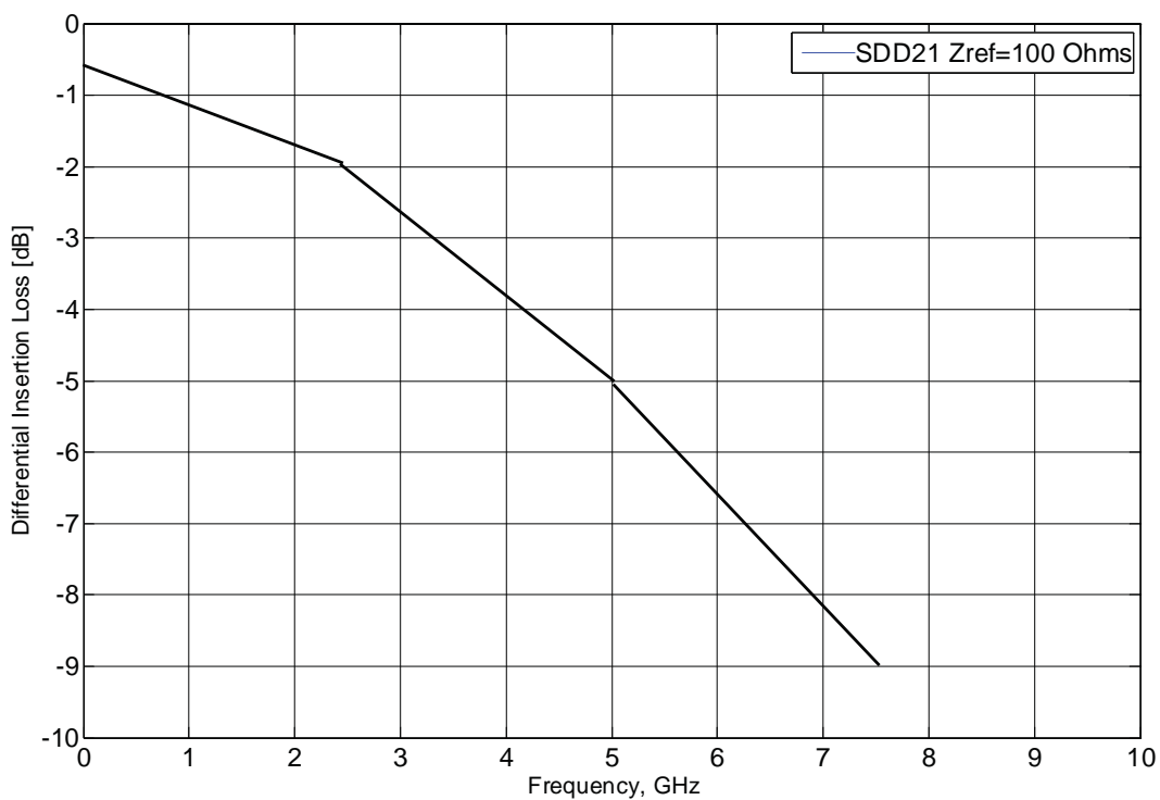
Figure 1: Illustration of differential insertion loss requirement.
