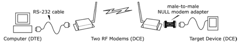
Figure B.3. Example of a Digi Radio Modem (DCE Device) connecting to another DCE device
