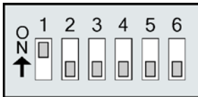
Figure 2.1. RS-232 DIP Switch Settings
