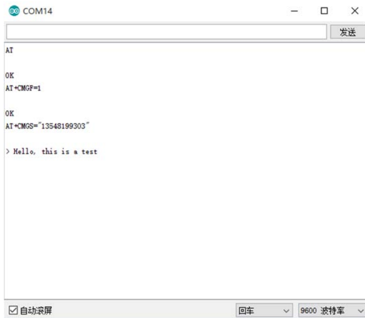
Arduino A6 GSM & GPRS Sending SMS
