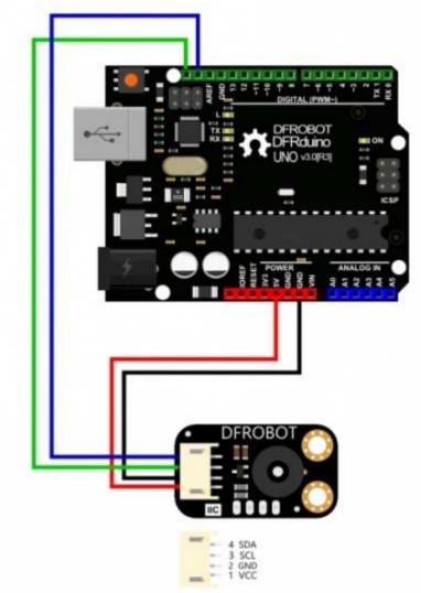
IR Thermometer Sensor-MLX90614 Wire Diagram
