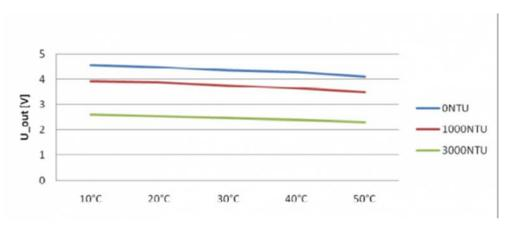
characteristic curve "Voltage ----Temperature
