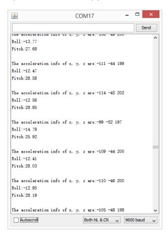
Result in Arduino IDE serial monitor
