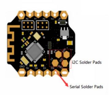
• 2. When soldering the Beetle to the Shield, make sure the orientation of the Beetle is correct so as to avoid connecting the wrong pins. The beetle should sit on the shield as pictured:
