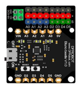
• 3. Please note that the Vcc pins for analog expansion pins is fixed at 5v. The Vcc pins for digital expansion pins is dependent on your power supply (5-8v DC)
