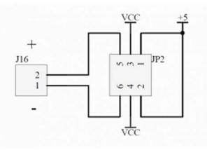
The middle pin is the shield VCC pin.
