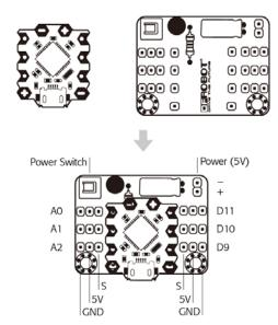
The Beetle can also be wired up individually. Thread the cables through holes according to IO port mapping. Some soldering will be needed for connection.
