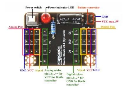
Beetle shield pinout (click to enlarge)
