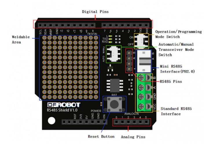
**Operation and programming mode switch**: To OFF, you can download the program for the Arduino controller. To ON , the shield will convert the UART to the RS485.
