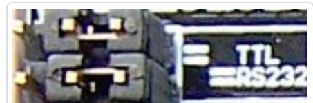
(/wiki/index.php/File:Sdb_v2.2_5.pr RS232/TTL Selection Jumpers
