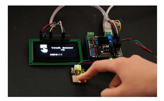
To ease the difficult of using this sensor, a Gravity Interface is adapted to allow plug&play. The IO expansion shield is the best match for this sound senor connecting to your Arduino. As this sensor can work at 3.3V which make it compatible with Raspberry Pi, intel edison, joule and curie.
