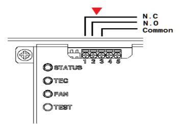
Alarm dry contact: (MAX. 60VDC 400mA or 125VAC, 400mA)
