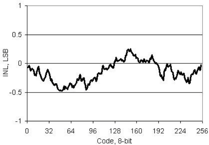
Figure 11-46. VDAC INL vs. Input Code, 1 V Mode
