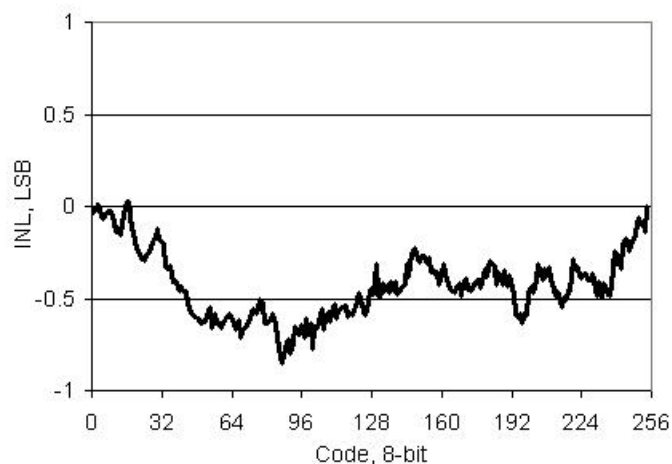
Figure 11-32. IDAC INL vs Input Code, Range = 255 \mu A, Source Mode
