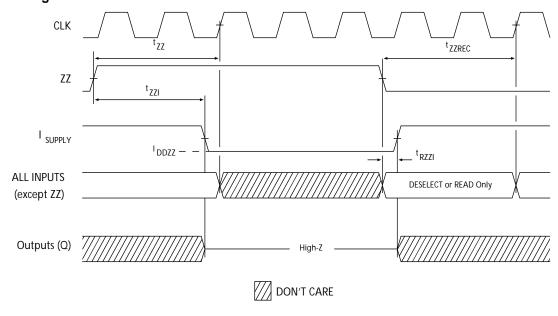
**Notes**35. Device must be deselected when entering ZZ mode. See Cycle Descriptions table for all possible signal conditions to deselect the device.
