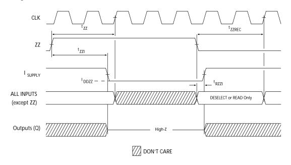
26. Device must be deselected when entering ZZ mode. See Cycle Descriptions table for all possible signal conditions to deselect the device. 27. DQs are in high-Z when exiting ZZ sleep mode
