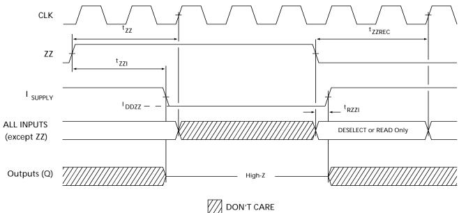
Notes: 21.Device must be deselected when entering ZZ mode. See truth table for all possible signal conditions to deselect the device. 22.DQs are in tri-state when exiting ZZ sleep mode.
