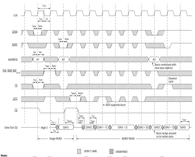
17. On this diagram, when  $\overline{CE}$  is LOW,  $\overline{CE}_1$  is LOW,  $CE_2$  is HIGH and  $\overline{CE}_3$  is LOW. When  $\overline{CE}$  is HIGH,  $\overline{CE}_1$  is HIGH or  $CE_2$  is LOW or  $\overline{CE}_3$  is HIGH.
