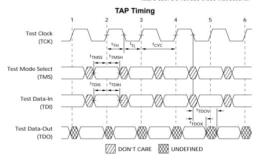
**TAP AC Switching Characteristics** Over the operating Range<sup>[9, 10]</sup>
