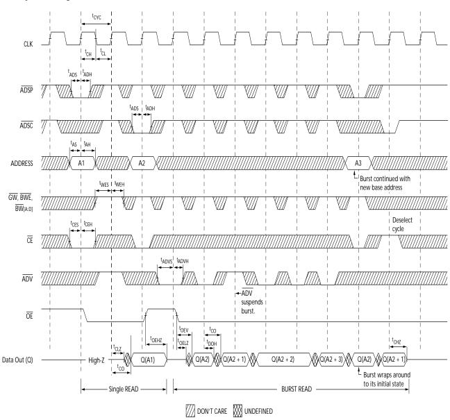
17. On this diagram when  $\overline{CE}$  is LOW,  $\overline{CE}_1$  is LOW,  $\overline{CE}_2$  is HIGH and  $\overline{CE}_3$  is LOW. When  $\overline{CE}$  is HIGH,  $\overline{CE}_1$  is HIGH or  $\overline{CE}_2$  is LOW or  $\overline{CE}_3$  is HIGH. 18. Full width write can be initiated by either  $\overline{GW}$  LOW, or by  $\overline{GW}$  HIGH,  $\overline{BWE}$  LOW and  $\overline{BW}_{[A:D]}$  LOW.
