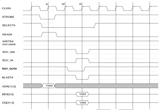
Use RWMODE = '01' to interface to a processor that has a read-write signal defined at R\_W (write is logic 0, read is logic 1). In this mode, the WRITE acts as R\_W and it is sampled
