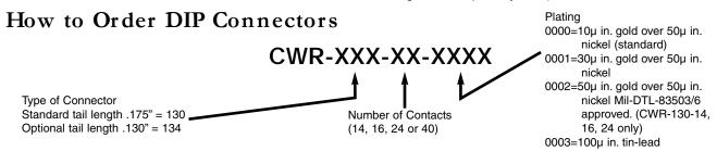
EXAMPLE: CWR-130-16-0002 is part number for a 16-pin DIP connector with .175 in. tails and 50µ in. gold over 50µ in. nickel contacts
