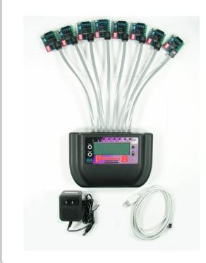
The Prime8 production programmer has eight high-speed ISCP<sup>™</sup> jacks for high volume programming. Ideal for production environments, it can operate as a stand-alone production programmer with its SD card reader, or with CCS software on the PC. Program up to 8 devices individually or concurrently.
